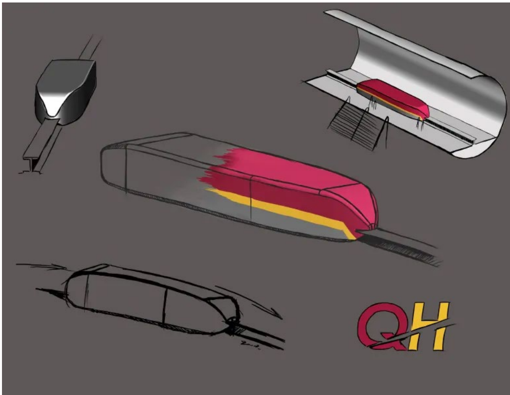
Figure 2: Initial design concept of Queen's Hyperloop pod
